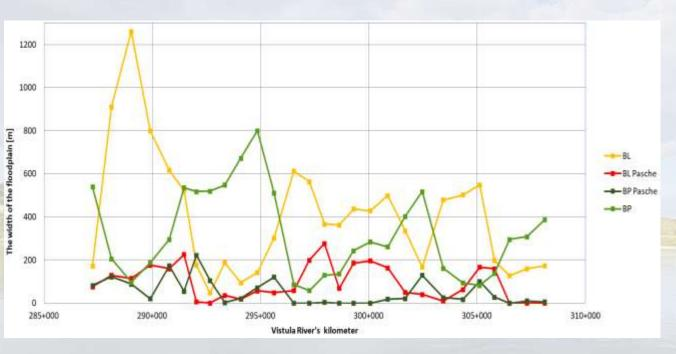
The width of the entire floodplain and the  $b_{II}$  zone according to the Pasche method, models 1D and 2D.
