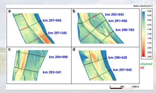
Spatial distributions of velocities in the cross-sections divided on the zones according to the Pasche method, Vistula river, discharge Q=4,000 m<sup>3</sup>s<sup>-1</sup>, a) compatible left bank, b) right bank incompatible, c) both banks incompatible, d) compatible both banks compatible.
