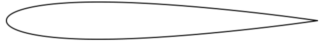
Fig 5: 2D NACA 0013 airfoil of total length 15 cm (NASA/Langley LS(1) )
