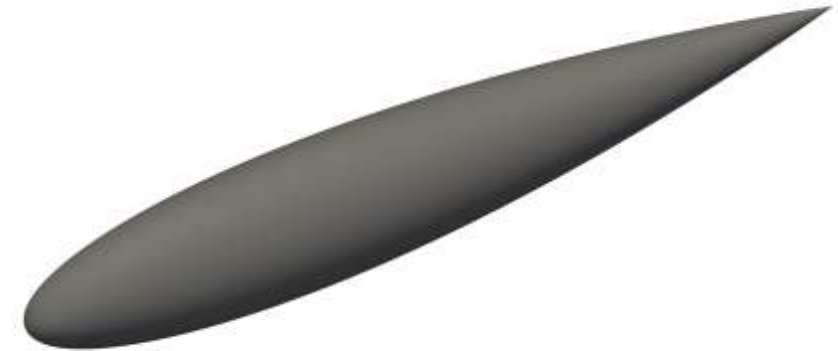
Fig 6: 3D axisymmetric body of NACA 0013 aerofoil representing fish
