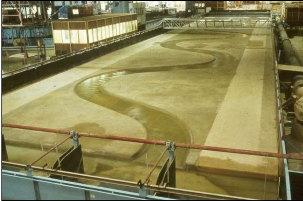
60° fixed bed channel Trapezoidal and change in shape Longitudinal dispersion
