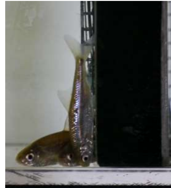
Fish fatigued while being impinged/resting on the rear grid
